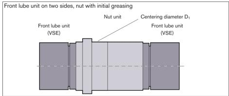
Mounting orientation of the front lube unit on nut types
