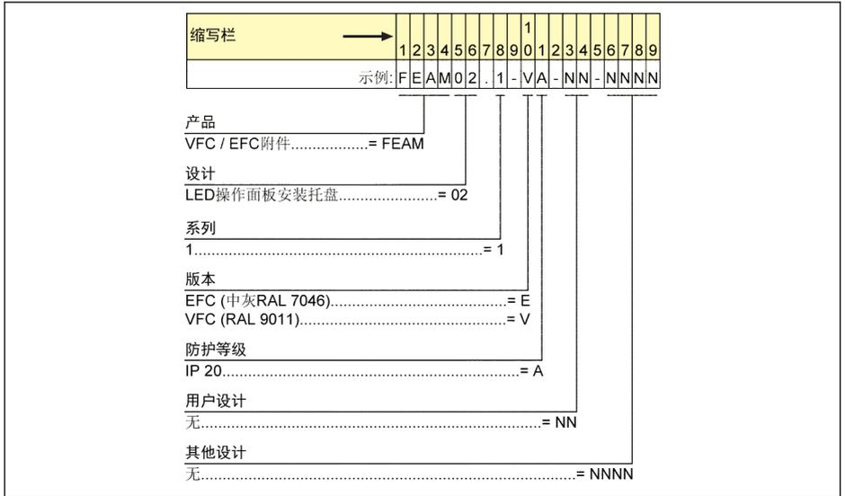
插图 18-3: 操作面板安装托盘类型编码
